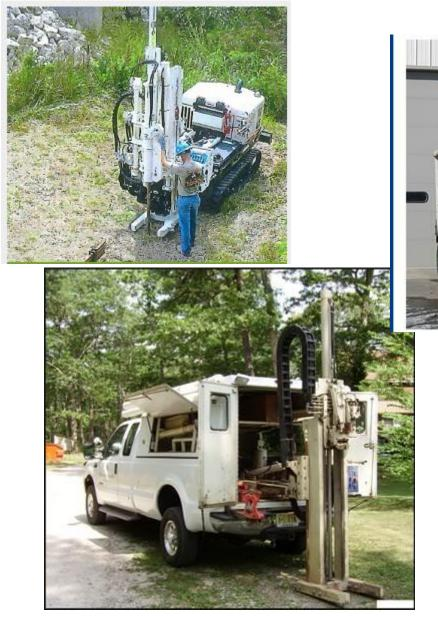
Pictures of the Geoprobe drill rigs.
